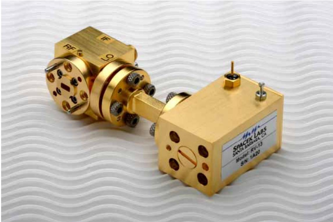
Spacek Labs Model RV-13 is a full-band receiver which downconverts all of V-Band (50-75 GHz) to an IF band from 1 to 26 GHz. The LO is derived from a free-running Gunn oscillator at 49 GHz. The RF port is WR-15 and the IF port is K" F". The LO bias is +7 volts @ 1A typ. This receiver can be used to extend the frequency range of a spectrum analyzer.
